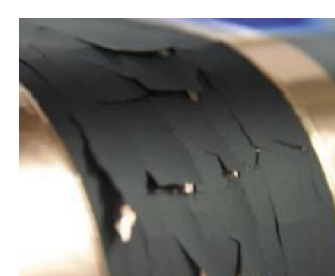
Delamination of electrode at too high drying rates
